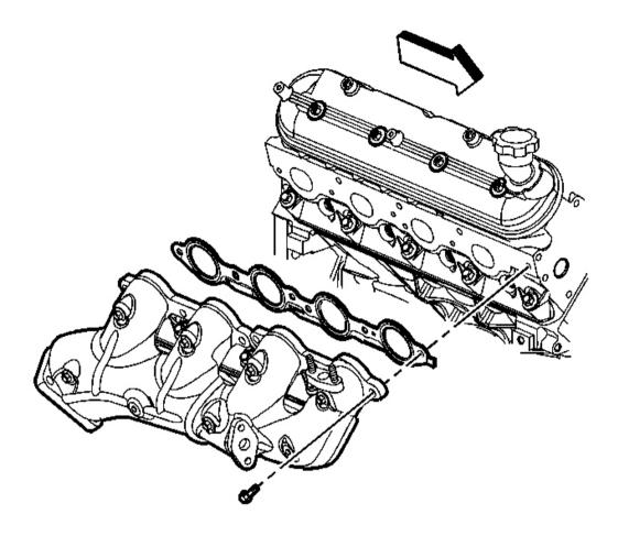
Fig. 11: Exhaust Manifold Bolts, Manifold & Manifold Gasket (Right) Courtesy of GENERAL MOTORS CORP.
