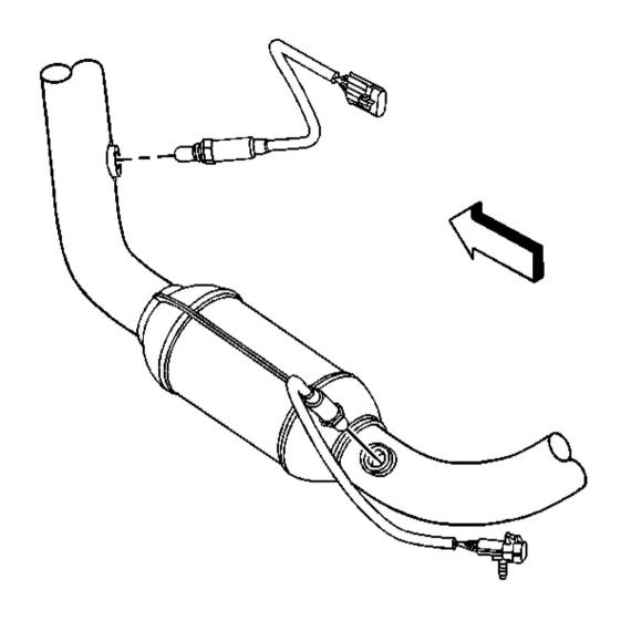
Fig. 28: Identifying O2 Sensors Courtesy of GENERAL MOTORS CORP.
