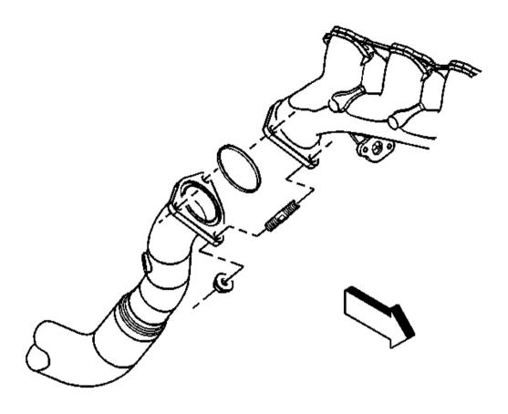
Fig. 20: Exhaust Manifold Pipe Nuts (Right) Courtesy of GENERAL MOTORS CORP.
