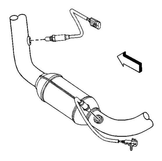
Fig. 29: Identifying O2 Sensors Courtesy of GENERAL MOTORS CORP.
