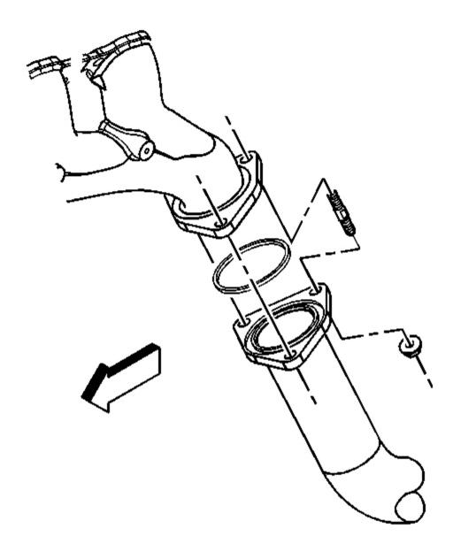
Fig. 1: Exhaust Manifold Pipe Nuts (Left) Courtesy of GENERAL MOTORS CORP.
