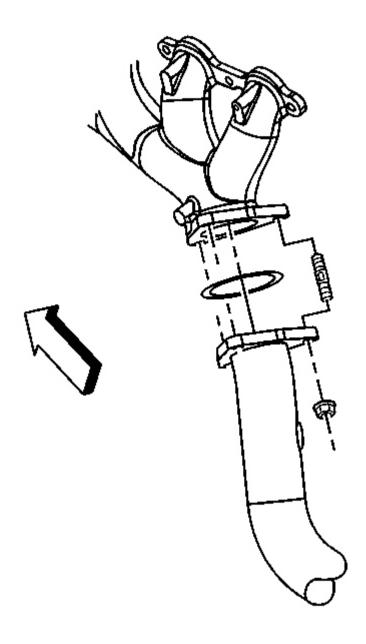
Fig. 26: Exhaust Manifold Pipe Nuts (Left) Courtesy of GENERAL MOTORS CORP.
