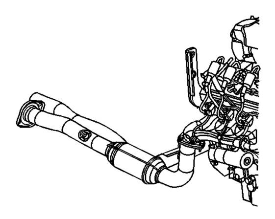
Fig. 27: Exhaust Manifold Pipe Courtesy of GENERAL MOTORS CORP.
