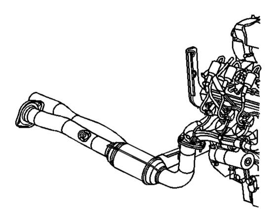
Fig. 16: Exhaust Manifold Pipe Courtesy of GENERAL MOTORS CORP.
