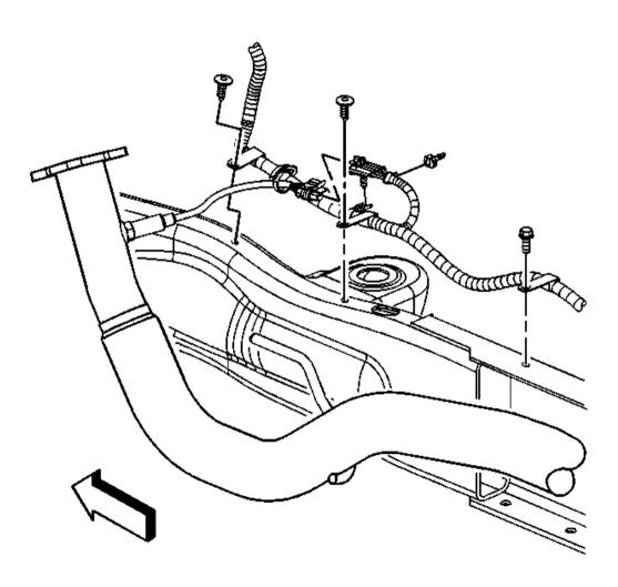
Fig. 13: View Of O2 Sensor Harness Courtesy of GENERAL MOTORS CORP.
