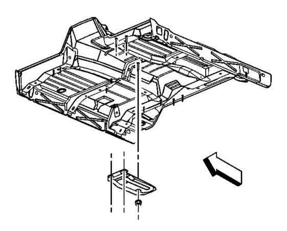
Fig. 38: Exhaust Front Heat Shield Nuts Courtesy of GENERAL MOTORS CORP.
