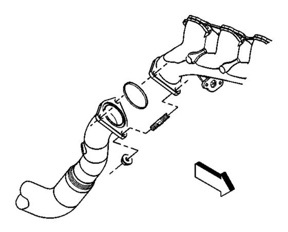
Fig. 17: Exhaust Manifold Pipe Nuts (Right) Courtesy of GENERAL MOTORS CORP.
