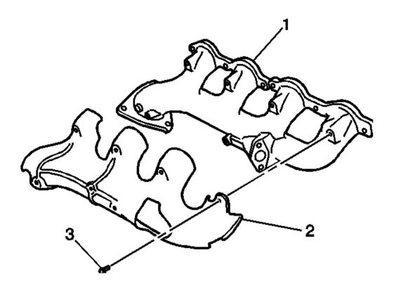
Fig. 9: Heat Shield Bolts, Heat Shield & Exhaust Manifold Courtesy of GENERAL MOTORS CORP.
