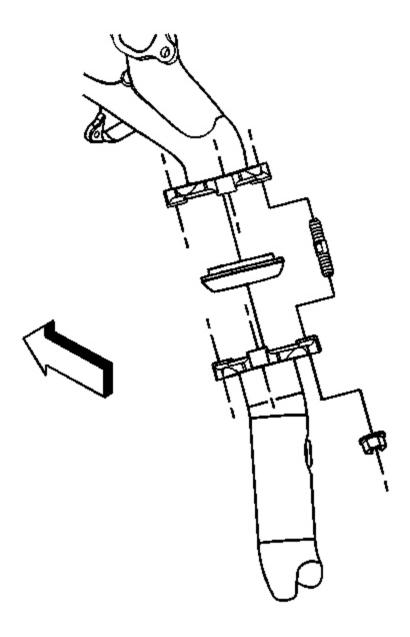
Fig. 12: Exhaust Manifold Pipe Nuts (Right) Courtesy of GENERAL MOTORS CORP.
