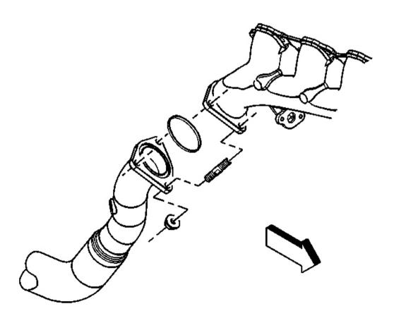
Fig. 23: Exhaust Manifold Pipe Nuts Courtesy of GENERAL MOTORS CORP.
