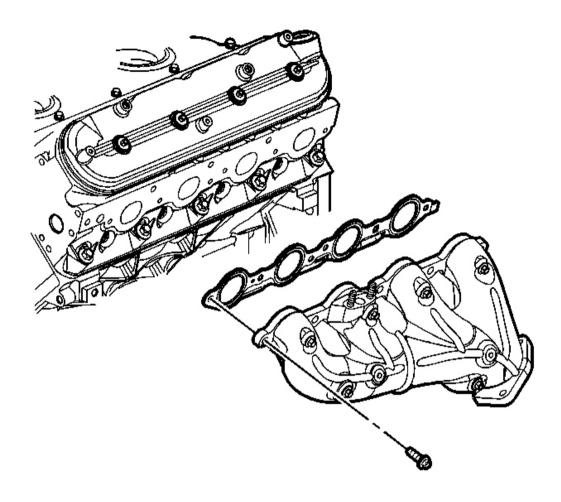
Fig. 2: Exhaust Manifold Bolts, Manifold & Gasket Courtesy of GENERAL MOTORS CORP.
