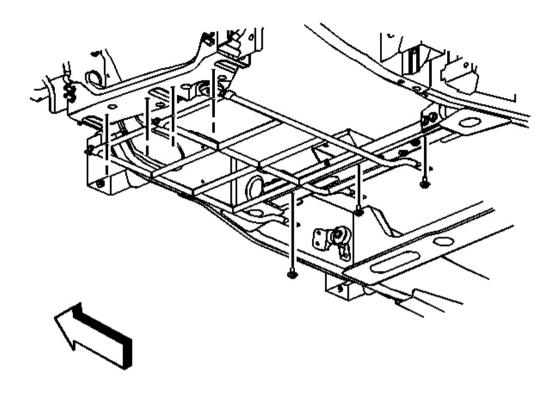
Fig. 33: Installing Catalytic Converter Guard Courtesy of GENERAL MOTORS CORP.
