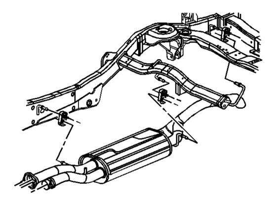
Fig. 36: Insulators & Muffler Hangers Courtesy of GENERAL MOTORS CORP.
