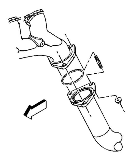
Fig. 6: Exhaust Manifold Pipe Nuts (Left) Courtesy of GENERAL MOTORS CORP.
