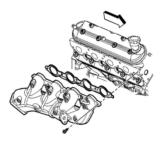
Fig. 8: Exhaust Manifold Bolts, Manifold & Manifold Gasket (Right) Courtesy of GENERAL MOTORS CORP.
