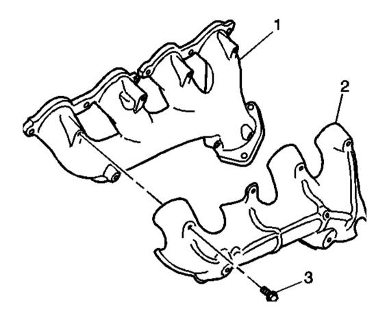
Fig. 4: View Of Heat Shield & Bolts (Left) Courtesy of GENERAL MOTORS CORP.
