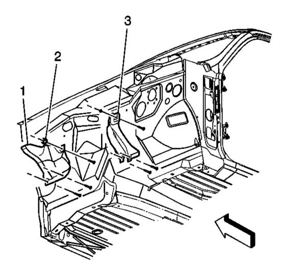
Fig. 43: Left Exhaust Heat Shield & Nuts (Dash Panel) Courtesy of GENERAL MOTORS CORP.
