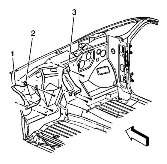
Fig. 44: Left Exhaust Heat Shield & Nuts (Dash Panel) Courtesy of GENERAL MOTORS CORP.
