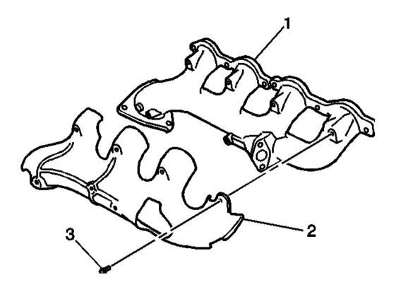
Fig. 10: Heat Shield Bolts, Heat Shield & Exhaust Manifold Courtesy of GENERAL MOTORS CORP.
