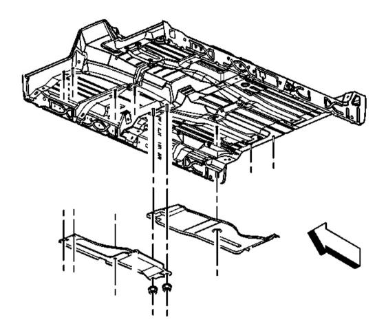
Fig. 39: Exhaust Heat Shield(S)
