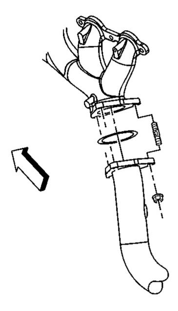
Fig. 31: Exhaust Manifold Pipe Nuts (Left) Courtesy of GENERAL MOTORS CORP.
