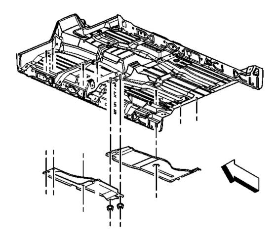
Fig. 41: Exhaust Heat Shield(S)
