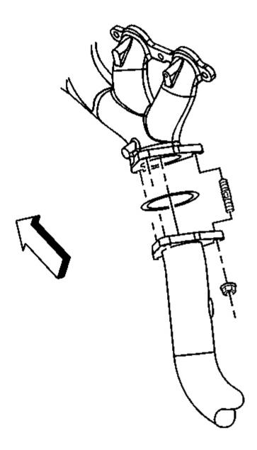
Fig. 22: Exhaust Manifold Pipe Nuts (Left) Courtesy of GENERAL MOTORS CORP.
