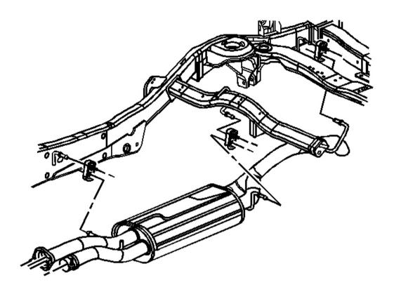
Fig. 35: Insulators & Muffler Hangers Courtesy of GENERAL MOTORS CORP.
