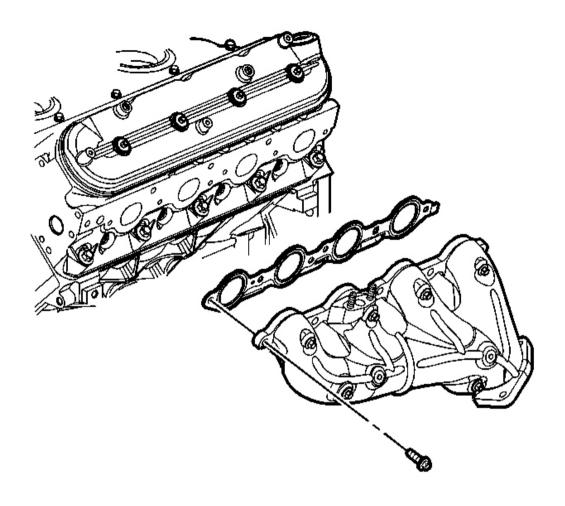
Fig. 5: Exhaust Manifold Bolts, Manifold & Gasket (Left) Courtesy of GENERAL MOTORS CORP.
