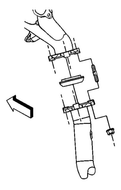
Fig. 7: Exhaust Manifold Pipe Nuts (Right) Courtesy of GENERAL MOTORS CORP.
