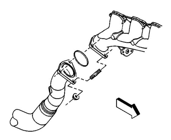
Fig. 14: Exhaust Manifold Pipe Nuts (Right) Courtesy of GENERAL MOTORS CORP.
