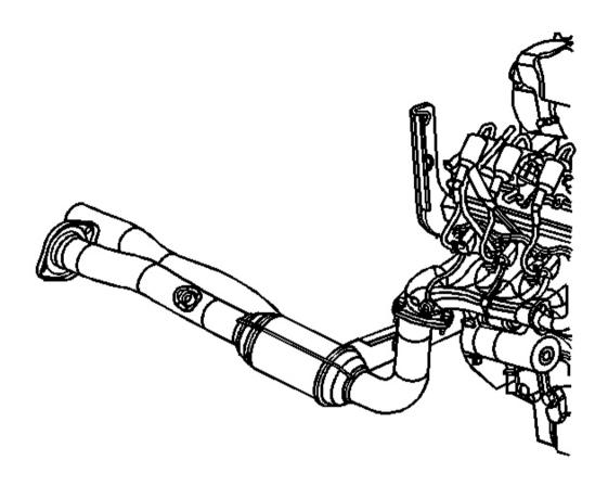
Fig. 30: Exhaust Manifold Pipe Courtesy of GENERAL MOTORS CORP.
