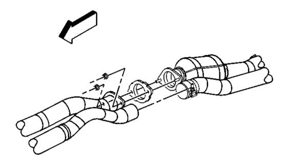
Fig. 37: Exhaust Muffler Nuts Courtesy of GENERAL MOTORS CORP.
