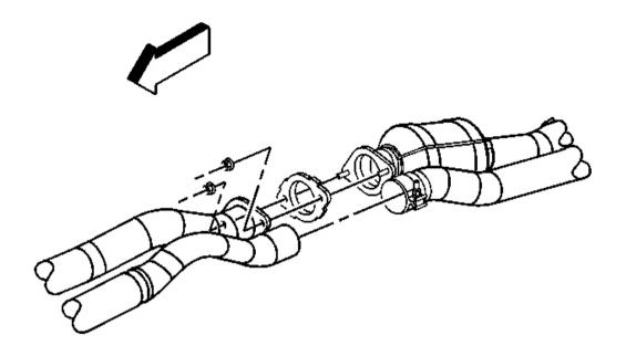
Fig. 34: Exhaust Muffler Nuts Courtesy of GENERAL MOTORS CORP.
