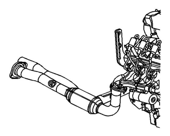
Fig. 15: Exhaust Manifold Pipe Courtesy of GENERAL MOTORS CORP.
