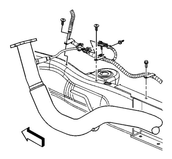
Fig. 18: View Of O2 Sensor Harness Courtesy of GENERAL MOTORS CORP.
