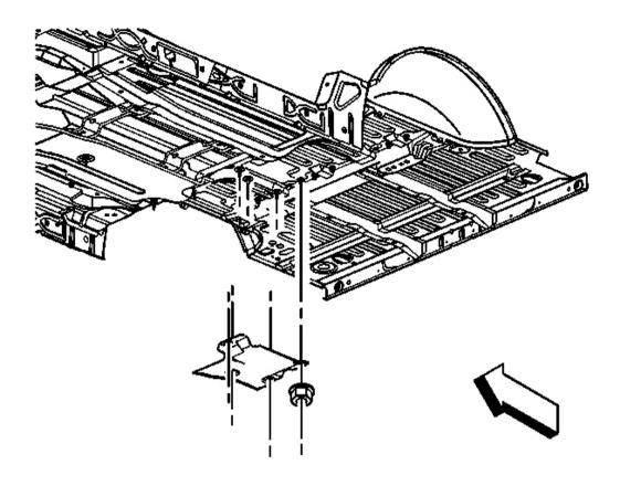
Fig. 40: Installing Exhaust Heat Shield To Studs Courtesy of GENERAL MOTORS CORP.
