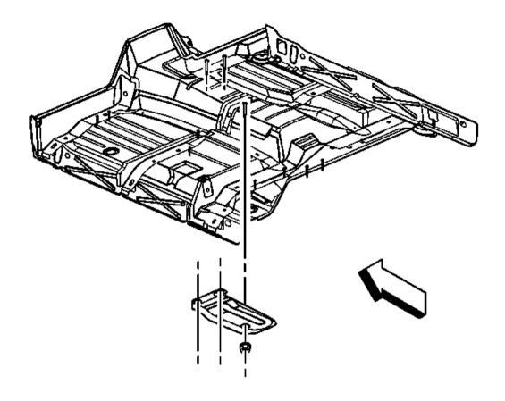
Fig. 42: Exhaust Front Heat Shield Nuts Courtesy of GENERAL MOTORS CORP.
